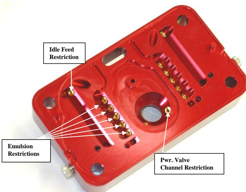
**Typical View of adjustable billet metering block with screw-in restrictions identified. Some not equipped with a screw-in power valve restriction.**
