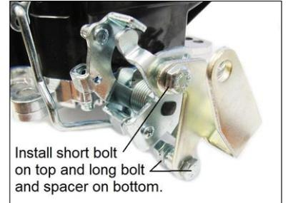
Install short bolt on top and long bolt and spacer on bottom.
