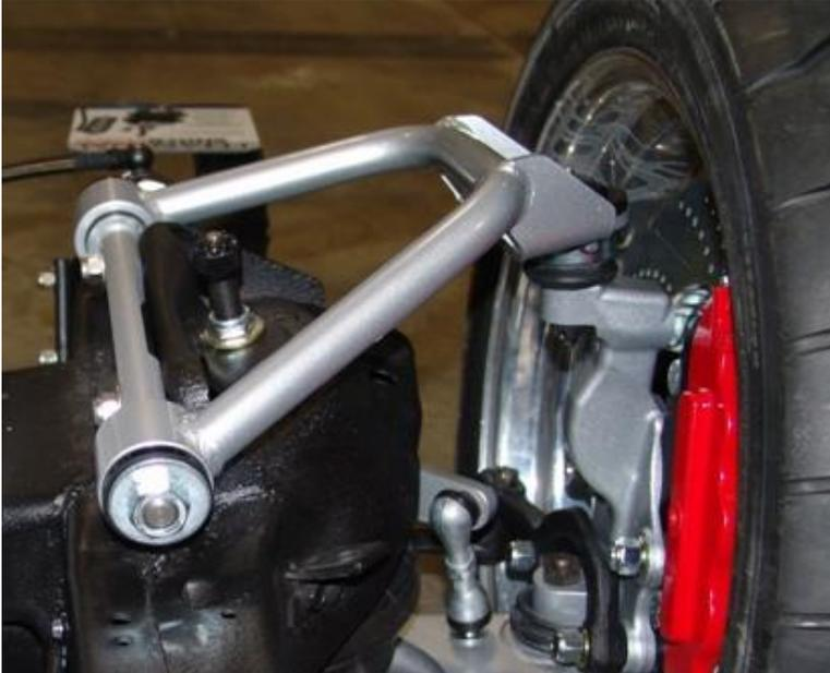
1. Fasten the upper arm to the frame using the supplied hardware. Reinstall the current alignment shims, but **vehicle must be realigned.**
