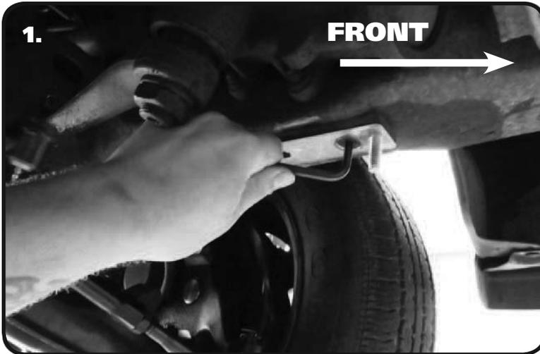
1. Attach the Adapter Plate to Frame positioned with the 3/8"-16 Stud to the Front of the Car and the Rear Hole aligned with the Rear OEM Hole. The Adapter Plate is attached to the Frame using a M10-1.5 x 30 Flat Head Bolt and Red Loctite. Apply Red Loctite to the proper Bolt and insert it through the Adapter. Thread the Bolt into the Front OEM Hole and tighten.
