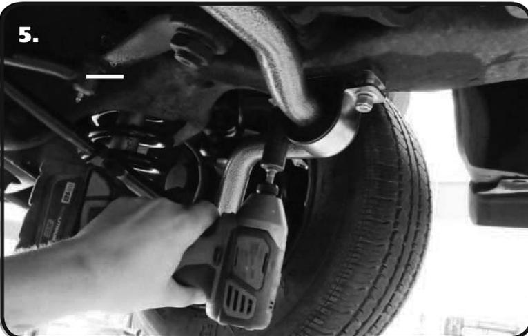
5. Slide the SwayBar into position on the Car. The SwayBar Arms will be above the Tie Rods. Slide the Front Hole of the SwayBar Bushing onto the 3/8" -16 Stud. Hold it in place with a 3/8" SAE Flat Washer and 3/8" -16 Nylok Nut. Install a 3/8" Lock Washer and 3/8" Flat washer on the M10-1.5 x 30 Hex Bolt and insert it into the rear mounting hole on each side. Do **NOT** Complete tighten the Hardware. It will be left partially loose until the End Links are installed.
