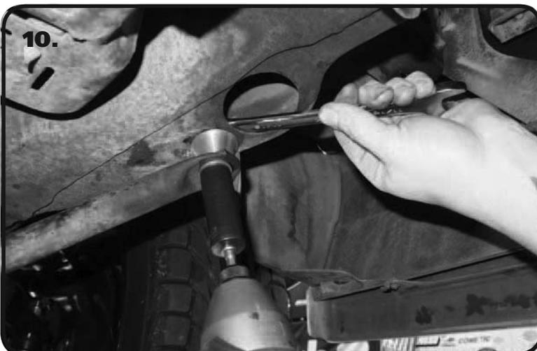
**10.** Tighten all of the mounting hardware. You can get a wrench on the front mounting nut through the large hole.
