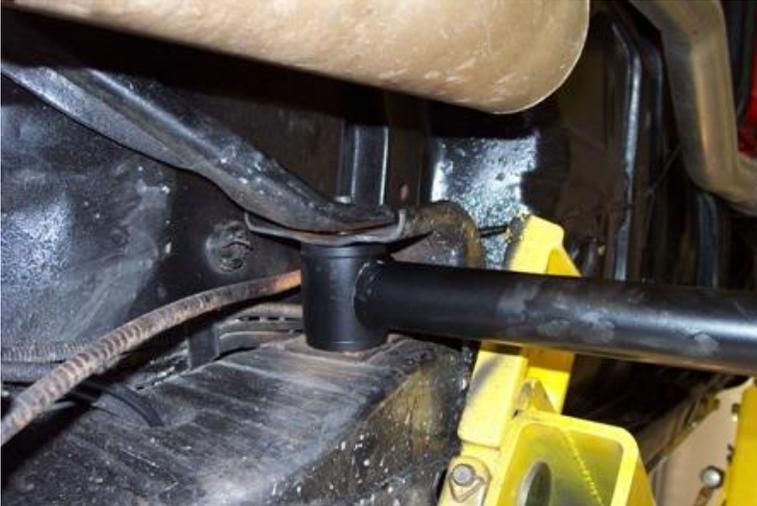
1. Remove the sway bar (if equipped) and factory lower trailing arm. Do one side at a time to keep the axle from rotating.
