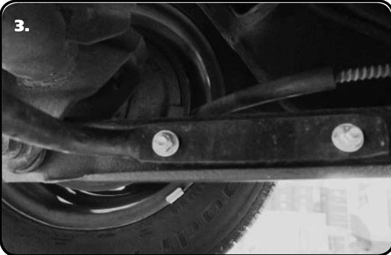
3. Slide the bar in Place with the LOW part of the bar down. Install a 7/16" washer on one of the 7/16"-14 x 3" Bolts and install one in each Front Hole to help hold it in place. Swing the SwayBar into position and insert the Rear Bolt/Washer. Tighten Hardware.
