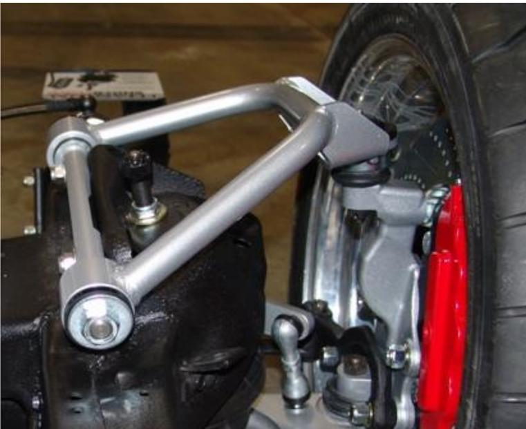
3. Drop ball joint down through upper arm. Slide ball joint boot over stud, then place boot retainer over the boot. Clamp assembly tight w/ the hardware supplied.
