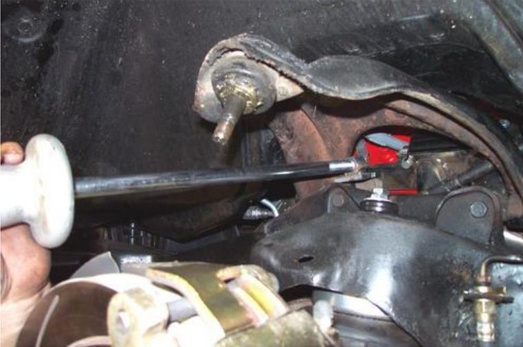
1. On some cars, to remove the upper control arm you must remove the bolts, which are pressed into the frame. We made this slide hammer adapter (a nut with a piece of angle iron welded to it) to aid in removing the bolts.
