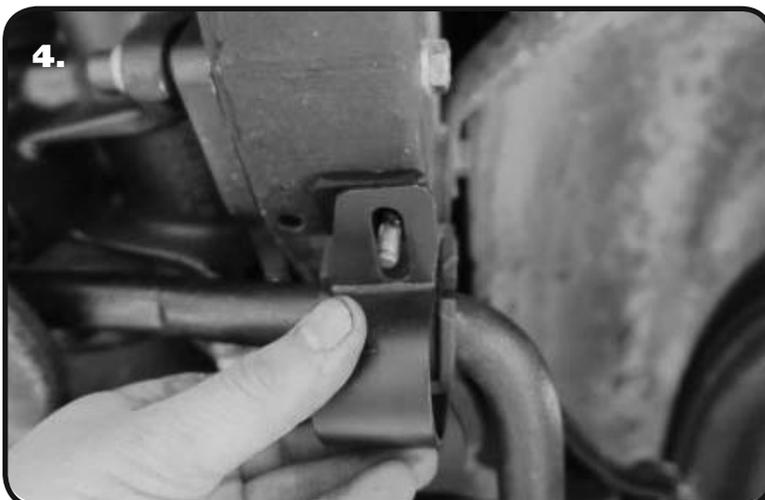
4. Slide the SwayBar into position on the Car. The SwayBar Arms will be above the Tie Rods, Idler Arm, and Pitman Arm. Install the bushing strap onto the bushing with the NARROW side to the outside of the frame. Install a 5/16" flatwasher and 5/16" nylok on each bolt sticking through the bushing strap. Do **NOT** Complete tighten the Hardware. It will be left partially loose until the End Links are installed.
